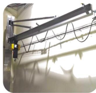
Stainless Steel Jib Crane with 45° Swivel
