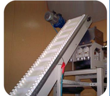
40m Long Belt Conveyor with Single Motor Drive
