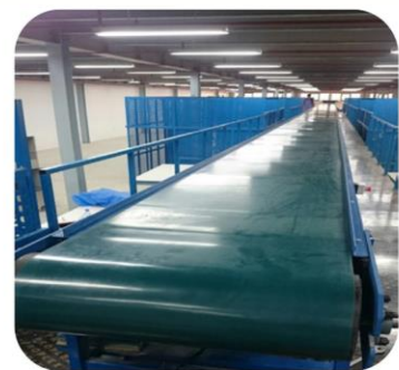
40m Long Belt Conveyor with Single Motor Drive
